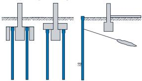
Ductile cast iron piles allow work under a limited height of 7.5 m or even 5.0 m and accessibility up to 2.5 m in width. Used in low headroom conditions, they offer impressive suitability for extension projects, rehabilitation of warehouses or strengthening of old foundations. The absence of excavated material and the low level of vibration makes their use all the more significant when the conditions of access and workspace are difficult.
