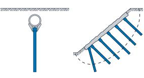
Underground pipe-laying on ductile cast iron piles represents an economic alternative to an expensive soil replacement method. The process allows the installation of the piles at different platform levels and an accurate vertical positioning of pipes, to durably prevent settlements.
