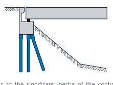
Thanks to the significant inertia of the continuous metallic tube and the easy installation of raked piles (inclination possible up to a 45 degree angle), ductile cast iron piles can support horizontal loads and high bending moments. They are particularly indicated for use in civil engineering works of appropriate dimensions (deep foundations of bridge piers and abutments for road and rail infrastructures) and in projects located in seismic zones.
