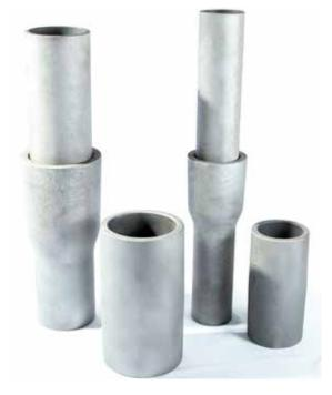
Designed as a very flexible system, the Plug&Drive© spigot and socket joint eliminates waste on pile lengths: excess lengths are fully reused as a starter piece for the next pile. Direct pile cutting-off to project level reduces time and cost of deep foundations, thus eliminating the traditional pile breaking off and allowing the immediate scheduling of concrete work.
