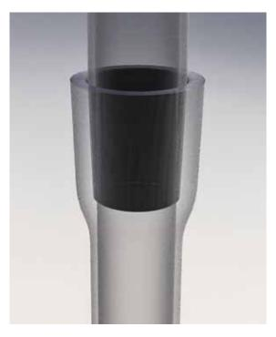
Shaft-grouted ductile iron piles are commonly driven to predetermined lengths in homogeneous or multilayer soils. The shaft grouting allows you to develop high skin friction and considerable tip resistance in both fine- and coarse-grained soils thanks to the creation of an interfingered soil/ pile interface and to the lateral soil displacement.
